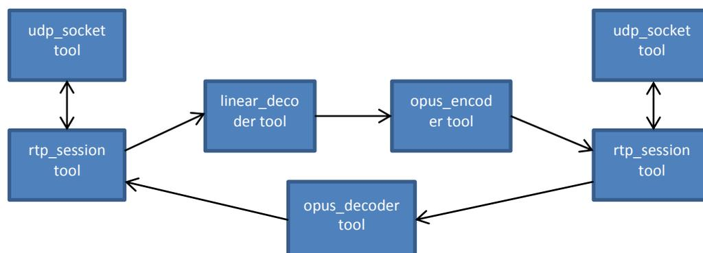
This script allows testing of NOF\_CHANNELS instances of the above tool configuration. Each channel represents full duplex trans-coder between linear and opus clients.
