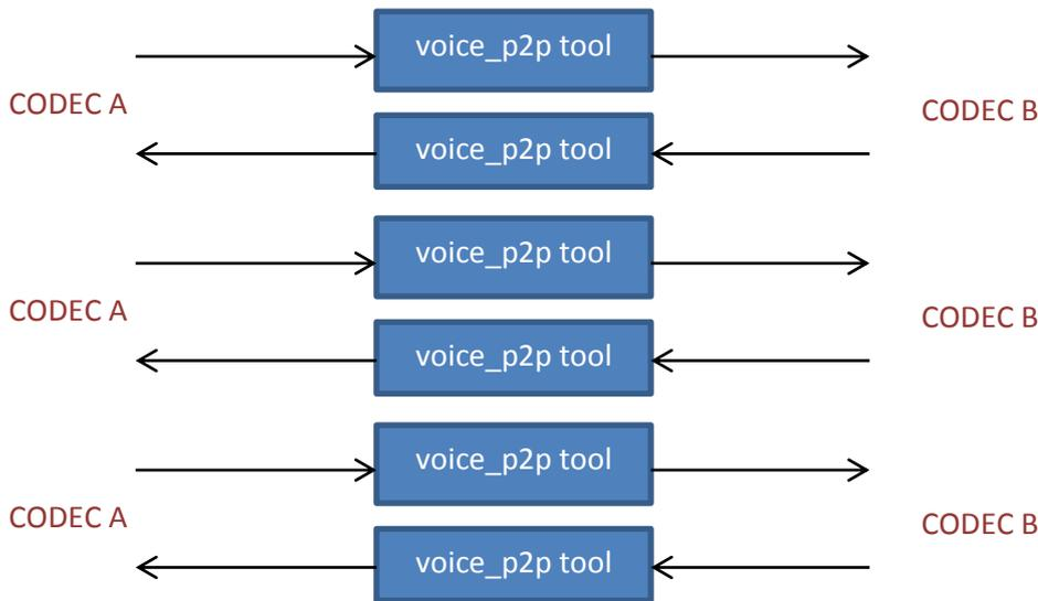
This is generic script for load testing of voice\_p2p trans-coding tools. It configures N voice trans-coder tools from codec A to codec B and N tools from codec B to codec A. In order to run this script, several parameters must be configured:
