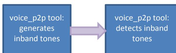
This script demonstrates inband DTMF detection functionality. This scenario contains 2 voice\_p2p tools: the first one generates inband DTMFs and the second one detects it and notifies the script.
