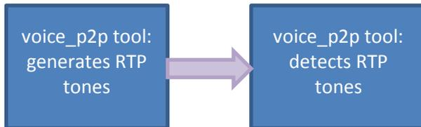
This script demonstrates RTP DTMF detection functionality. This scenario contains 2 voice\_p2p tools: the first one generates RTP DTMFs and the second one detects it and notifies the script.
