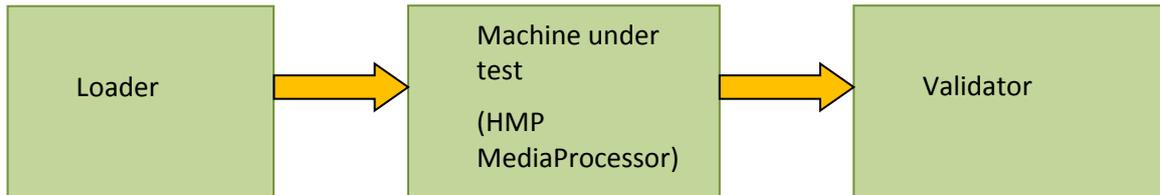
All 3 entities can be run on the same physical host, or can be divided into 2 or 3 different hosts, but for heavy load tests it is recommended to separate all 3 entities to 3 different hosts.
