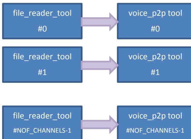
This script can be used for density testing in file play scenario. It creates required number of tools pairs when each pair contain file\_reader and voice\_p2p tools. In order to run this script
