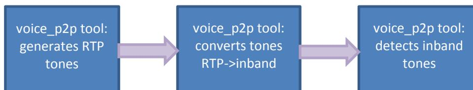
This script demonstrates conversion of RTP DTMF tones to inband DTMF tones. 3 voice\_p2p tools are created for this purpose. The first one generates RTP tones; its output is connected to the second tool's input. The second tool converts RTP tones to inband voice tones and sends it to its output which is in turn connected to the third tool's input. The third tool detects those inband tones and notifies the script.
