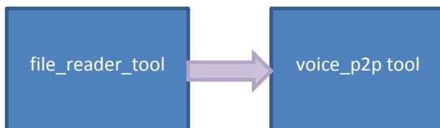
This script demonstrates file play functionality. It configures 2 tools: file\_reader and voice\_p2p. File reader tool receives a play list from configuration, reads corresponding files and passes its content to voice tool. The voice tool trans-codes the received voice and sends it to RTP destination.
