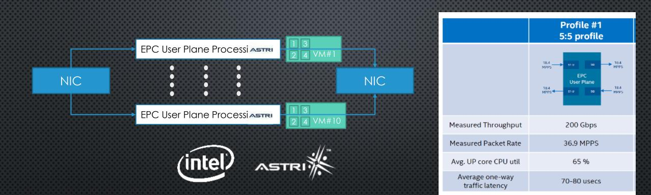
ASTRI: High Performance virtual EPC User Plane Processing stack Intel: Intel Scalable Processor Platform + NIC: load distribution to VMs with linear scale up
