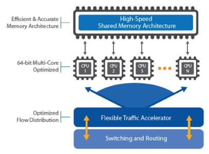
processing of traffic. For management functions, ACOS allocates a dedicated CPU for management purposes. As a result, administrators can reach devices and perform supervisory and health checks even under peak traffic conditions. The separation of management functions onto a separate core enables management flexibility and improves overall system robustness.
