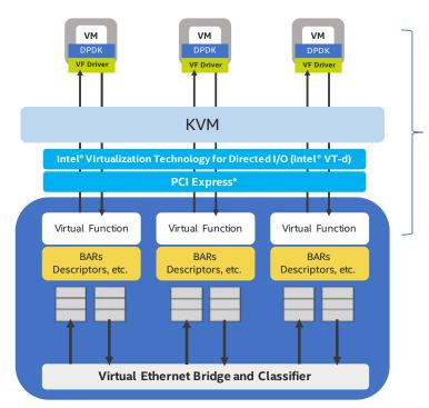
Networking applications running in VMs can directly access Ethernet controller ports without hypervisor (e.g., KVM) intervention
