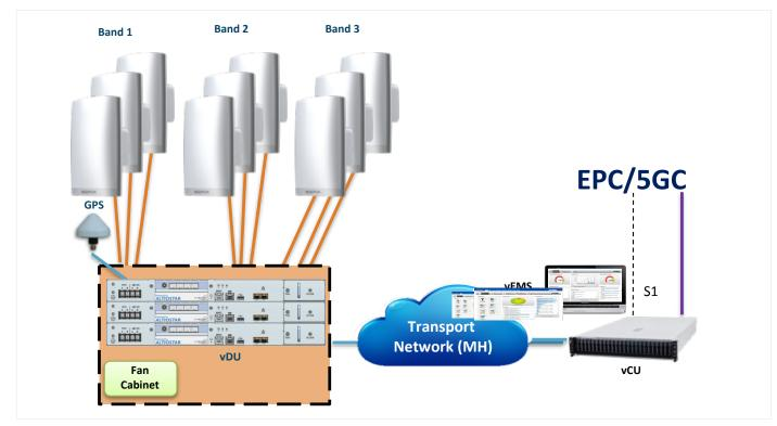
Figure 2. Higher performance server hosts vDU that can process data load of multiple RRHs.
