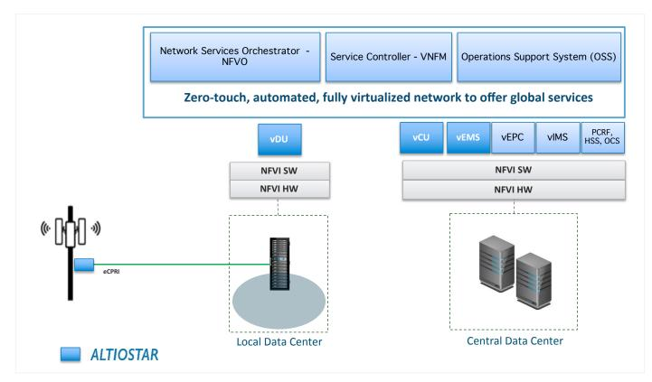
Figure 1. Model 1 diagram with vDU in a local data center that is served by a fiber-optic transport network.<sup>2</sup>
