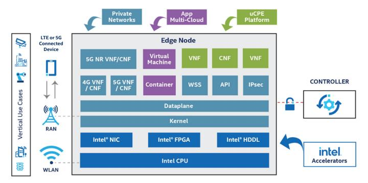
Figure 1. High level architecture of the Intel® Smart Edge platform
