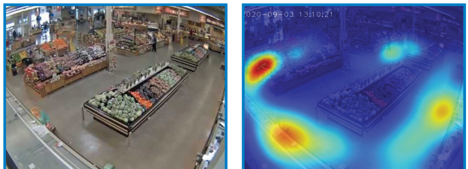
Figure 1. Video images (left) transformed into a shopper-presence heatmap (right).
