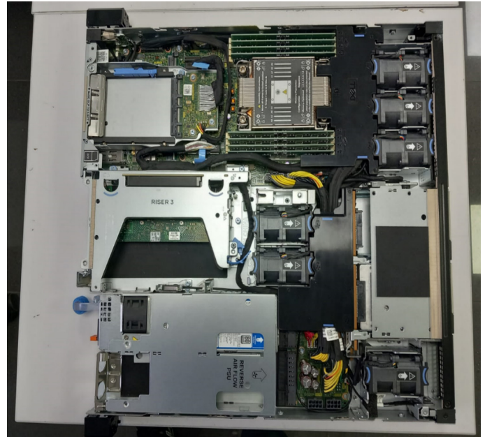
Figure 2. Air-cooled Dell PowerEdge XR5610 server
