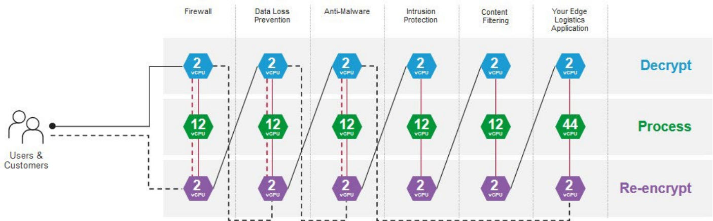
Figure 1. Virtualization and SSL Orchestration showing each step of web service delivery before activating QAT
