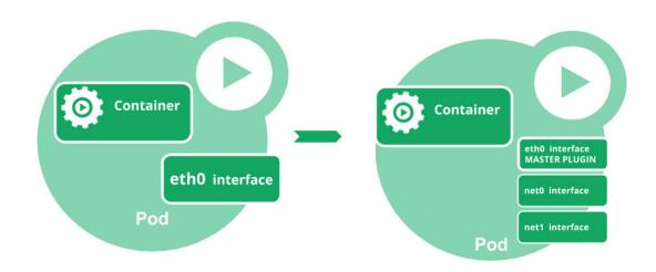
**Figure 3.** Before and after adding a Multus Plugin to the CNI (Image Source <u>here</u>)
