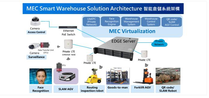
Figure 2. MEC-based smart warehouse solution architecture.<sup>1</sup>
