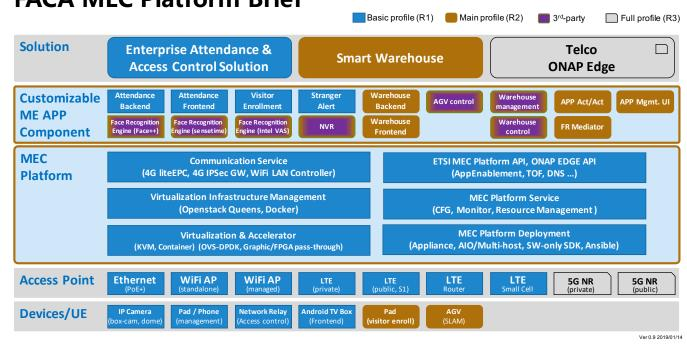
Figure 1. Block diagram of MEC solution developed by the Foxconn Advanced Communication Academy (FACA).<sup>1</sup>
