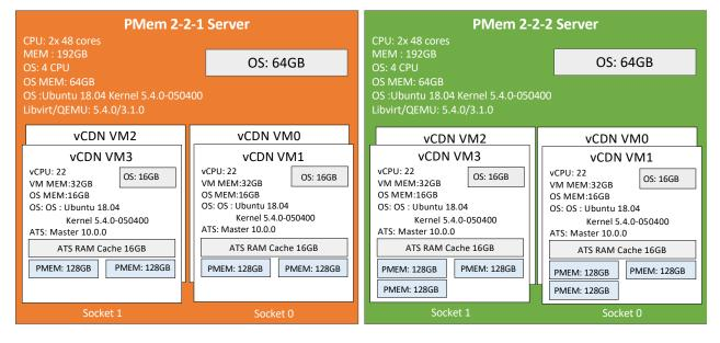
Figure 10. Test Topology: DUT1 and DUT2
