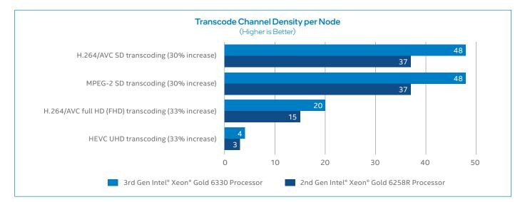
Figure 4. Improvements in channel density for various transcoding workloads.<sup>1</sup>
