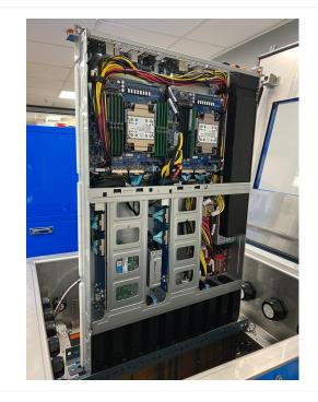
Figure 4. Intel 2U modular server chassis
