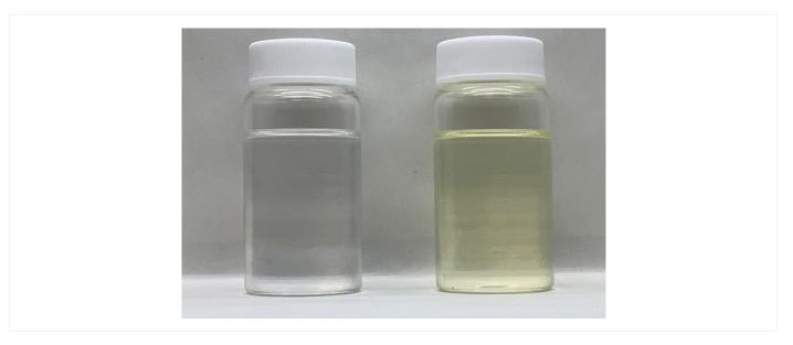
Figure 11. New ENEOS immersion cooling fluid (left) and general lubricant base oil (right)
