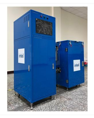
**Figure 2.** The 15kW cooling reference design solution includes CDU on left and 12U immersion tank on the right
