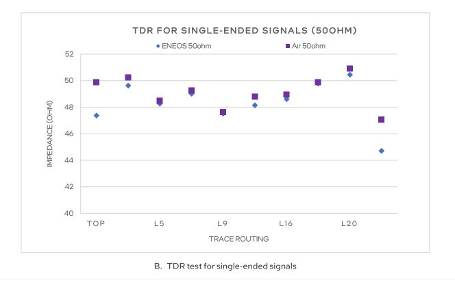
Figure 6. PCB TDR test comparison
