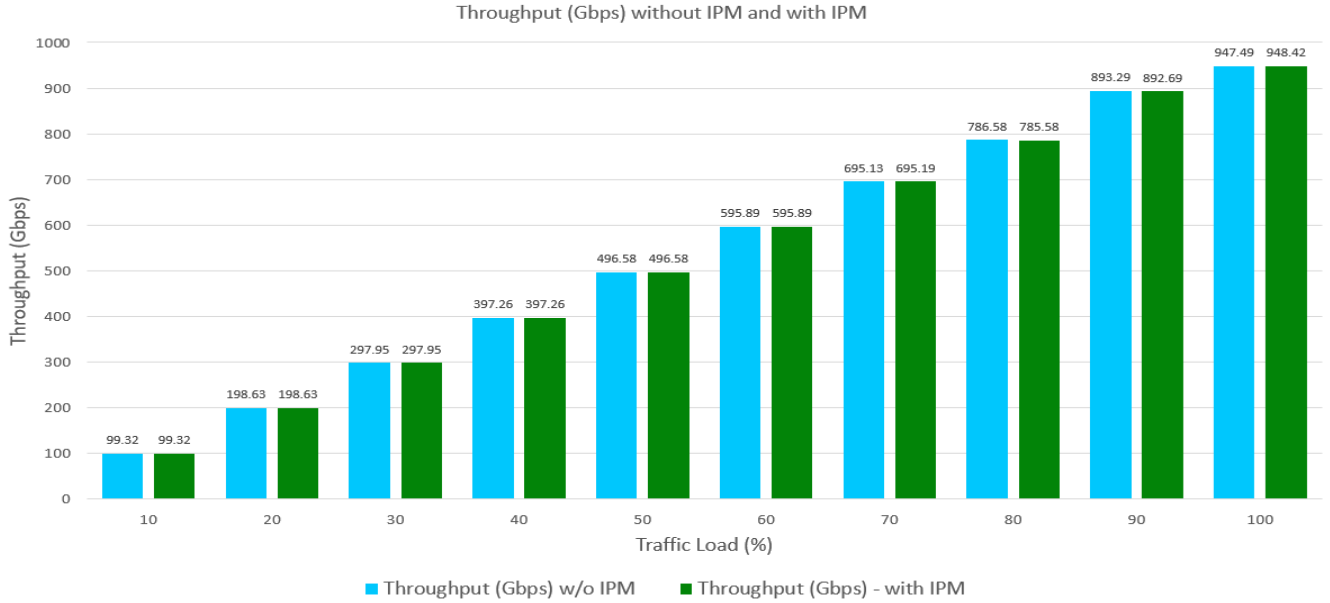
Figure 2. FlexCore 2.0 UPF Throughput (Gbps) with and without IPM 1,2
