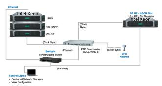
Figure 14. L1 Bypass mode lab setup
