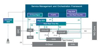
Figure 13. The Capgemini Engineering RATIO ORAN-based architecture
