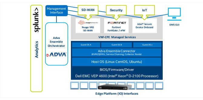
Figure 1. uCPE reference configuration block diagram.
