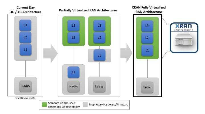
Figure 1. Three approaches to delivering the RF Source components in the RAN.<sup>6</sup>
