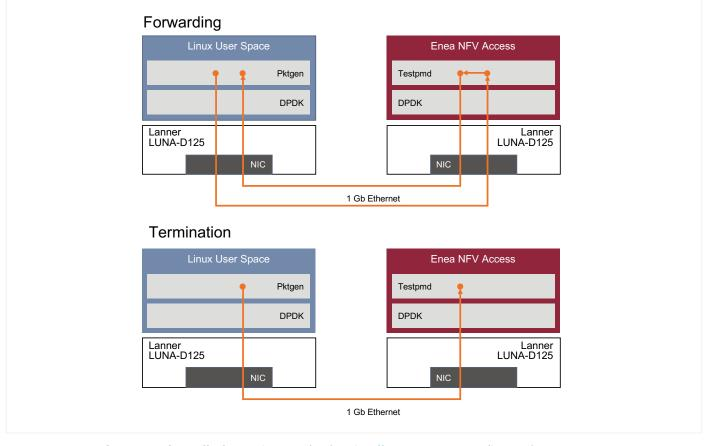
Figure 2. Test configurations for traffic forwarding test (top) and traffic termination test (bottom).<sup>4</sup>
