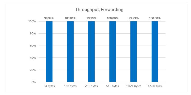
Figure 3. Throughput results from tests on LUNA-D125 with Enea NFV Access.<sup>3</sup>
