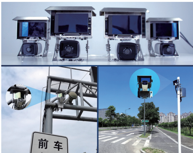
Figure 5. Leishen® All-in-One Roadside Sensing Equipment (Lidar & Camera).
