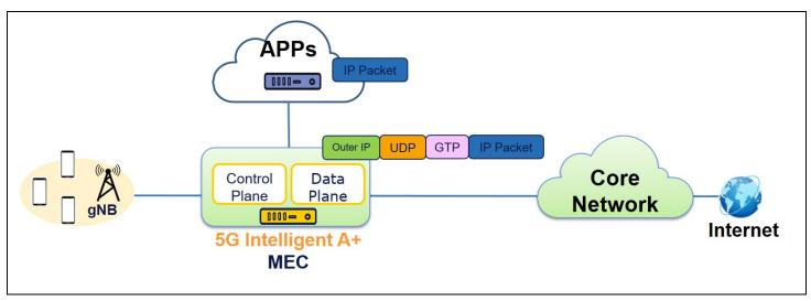
Figure 2. Components of Chunghwa Telecom\* 5G Intelligent A+
