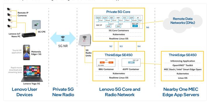
Figure 1. Sample deployment with containerized 5G BBU, 5G Core, and MEC converged at edge.
