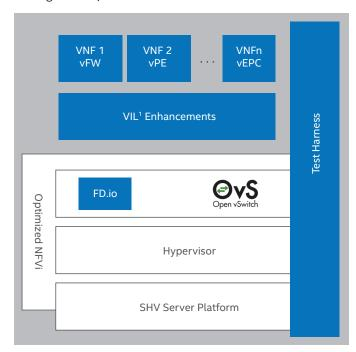
'VIL - VNF Infrastructure Libraries includes DPDK Optimized NFVi - DPDK based Open vSwitch\* (OVS). Refer to the Test Harness for KPIs for details: https://builders.intel.com/docs/ networkbuilders/network\_services\_benchmark\_NSB\_test\_ harness.pdf
