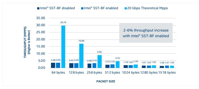
Figure 7. PROX l2fwd throughput results while 1 high priority core was pinned to OVS
