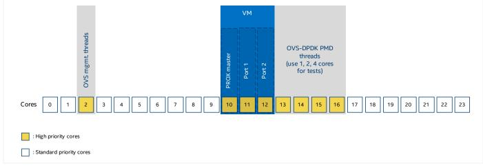
Figure 4. Core Configuration for OVS-DPDK and VM
