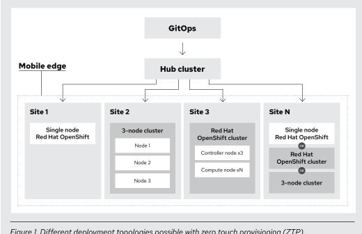
Figure 1. Different deployment topologies possible with zero touch provisioning (ZTP).
