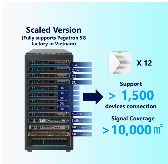
Figure 2. Pegatron 5G Scaled Version private 5G solution.
