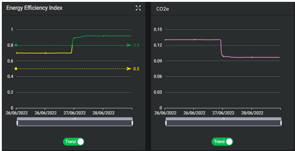
Figure 7. Stress-ng Workload Server EEI and Carbon Emissions in Foresight Optima DC+™ Dashboard
