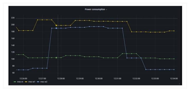
Figure 14. Power Consumption of the Node (mec-w2) when it is scaled-in and scaled-out
