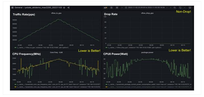
Figure 12. OS based Application Power Management Results (P-state enabled/Turbo-Off)
