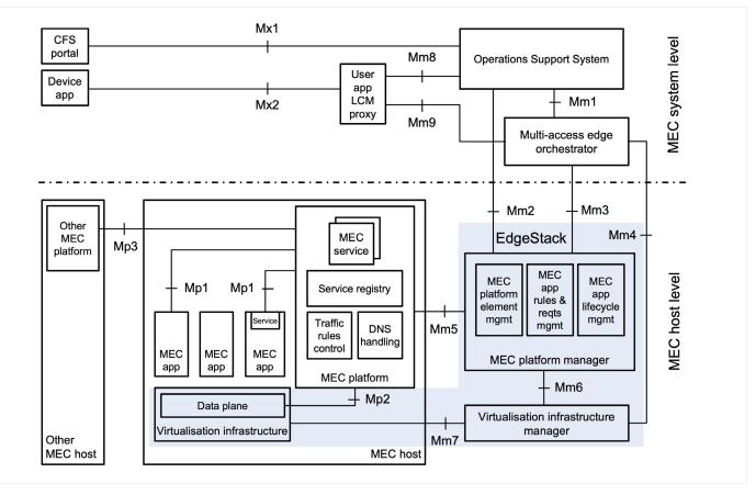
Figure 1. ETSI MEC Reference Architecture and SKT EdgeStack
