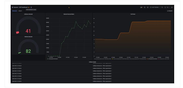
Figure 10. Power Consumption of ITM VM After RTSP Stream Coming from External Traffic Generator
