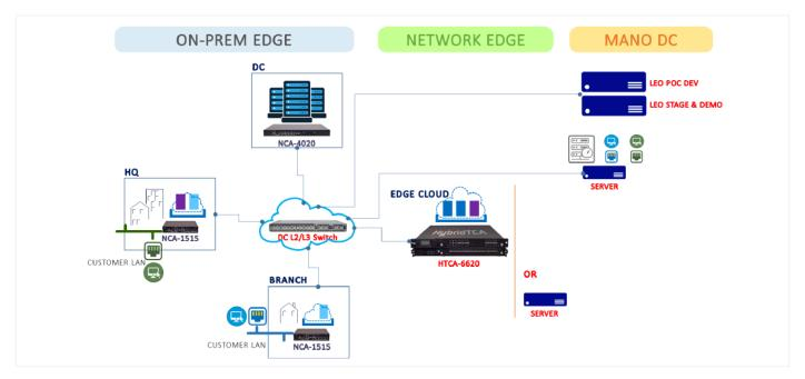
Figure 4. NEAT Lab configuration.
