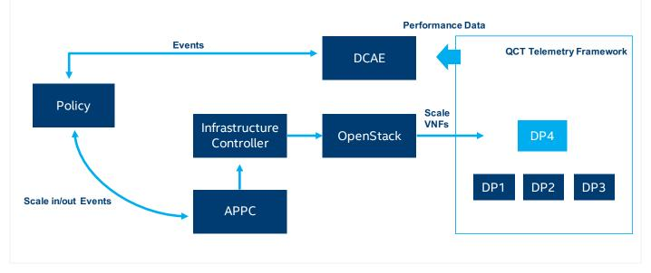
Figure 6. Auto-scaling closed loop automation—run time.
