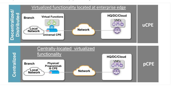
Figure 2. Comparison of centralized vs. decentralized approaches to virtualization.
