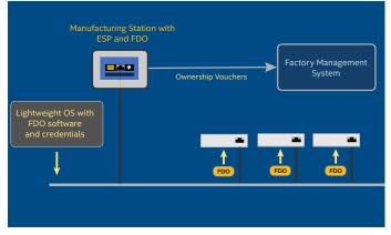
Figure 2. ESP Manufacturing environment to initialize FDO with a lightweight OS
