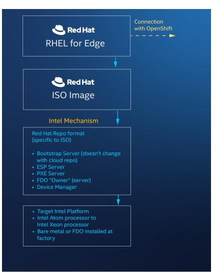
Figure 5. Installing the ISO image to the target Intel platform
