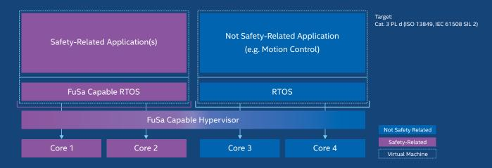
Both safety & not-safety workloads consolidated onto a single computing platform
