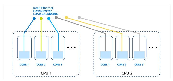
Figure 7. The ESP packet distribution with Intel Ethernet Flow Director
