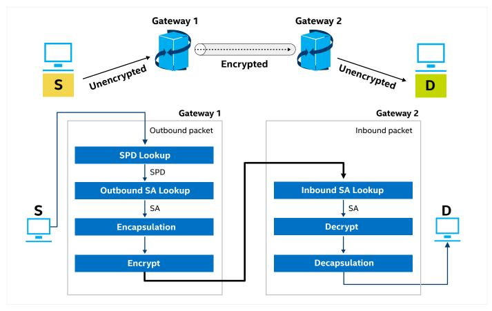
Figure 8. The encryption/decryption process in IPsec VPN
