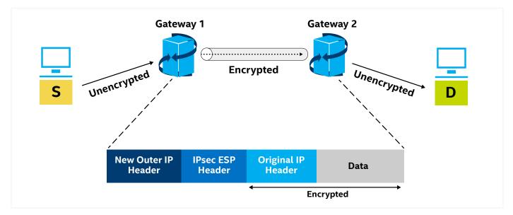
Figure 1. The components of IPsec VPN tunnel
