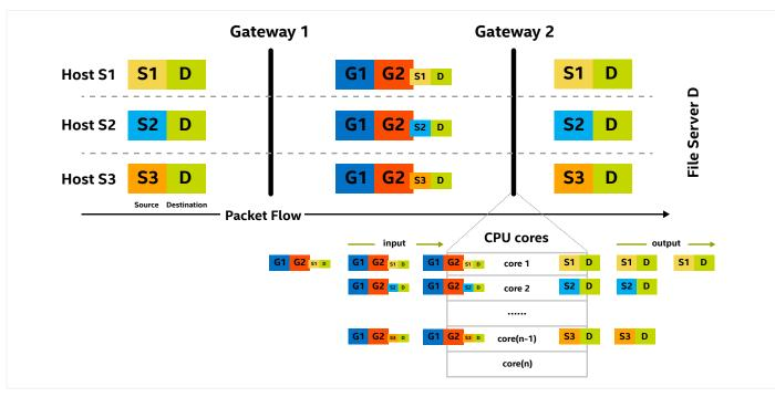
Figure 3. The distribution process of the ESP packet
