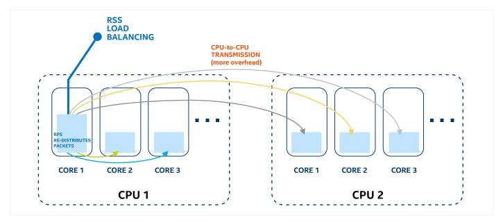
Figure 6. The packet distribution with RPS
