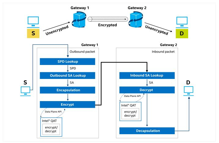
Figure 9. The encryption/decryption process using Intel® QAT
