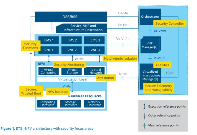
The cost and performance advantages of virtualization also introduce new security challenges that require a new approach to developing the layers of security, attestation, and domain isolation. Figure 1 overlays the traditional ESTI-NFV architecture with identified security-related focus areas. These are the broad areas of focus across industry standards bodies, open source consortia, and within Intel to address security across the NFVI and VNF stacks.
