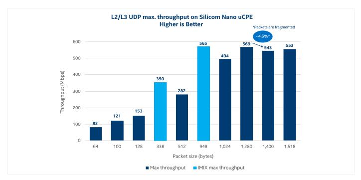
Figure 5. Layer 2/3 test results for Silicom Nano uCPE.<sup>1</sup>
