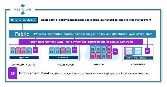
Figure 1. vArmour system architecture<sup>1</sup>
