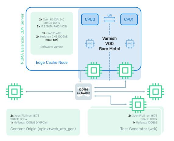
Figure 1: Bare metal CDN test environment
