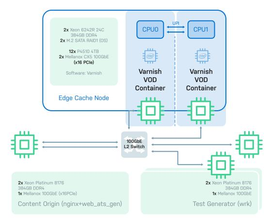
Figure 2: Containerized CDN test environment
