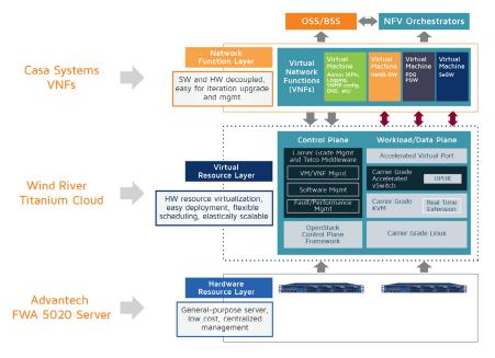
Figure 1. Virtual security gateway system architecture
