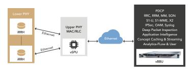
Figure 7. Altiostar vRAN architecture: Functional split options
