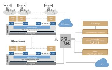
Figure 6. NFV architecture on commercial off-the-shelf hardware
