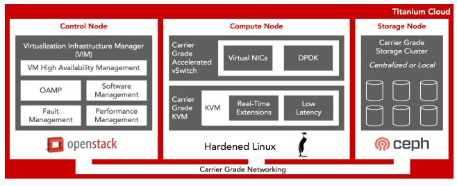
Figure 1. What's included in Wind River Titanium Cloud\*1
