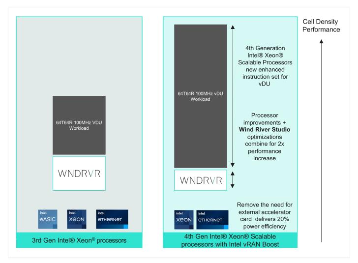
**Figure 5.** Performance results from the Wind River Studio tests (higher is better) The 3<sup>rd</sup> Gen Intel<sup>®</sup> Xeon<sup>®</sup> Scalable processors support 20 radios on two cores, whereas the 4<sup>th</sup> Gen Intel<sup>®</sup> Xeon<sup>®</sup> Scalable processor supports 32 radios on one core.
