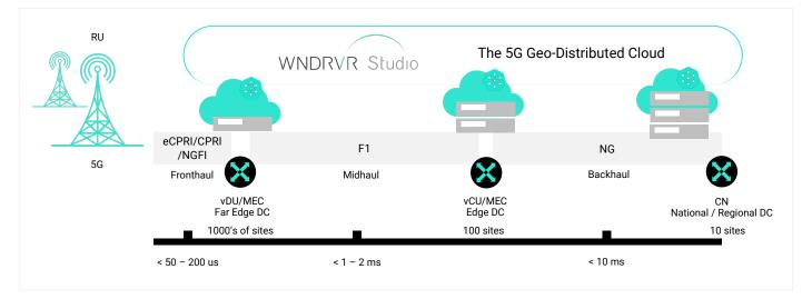
Figure 2. Wind River Studio Cloud Platform deployed as Individual distributed clouds with centralized management.
