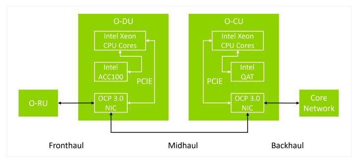
Figure 3. Hardware setup of Wiwynn 5g SA sub-6 GHz O-DU and O-CU.
