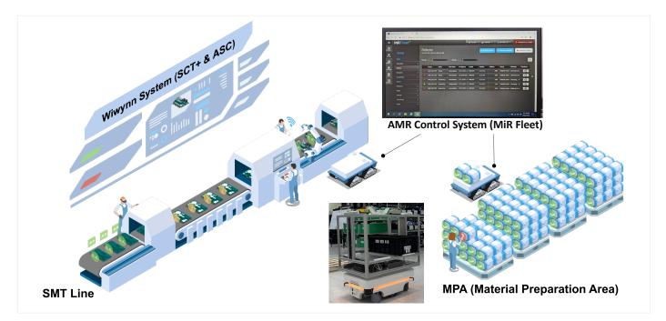
Figure 7. Architecture of Wiwynn AMR in in the Wiwynn smart factory.
