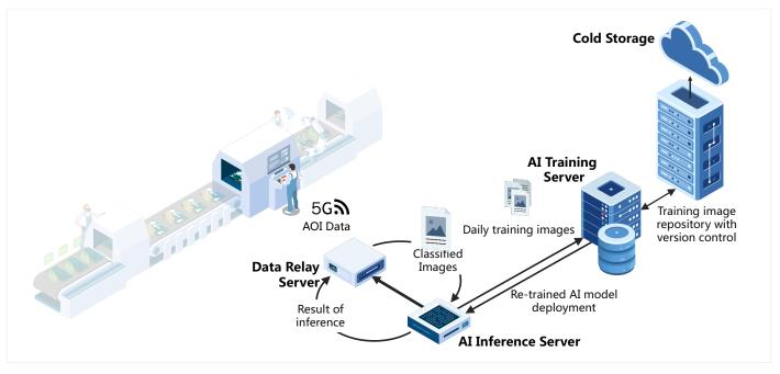
Figure 5. Architecture of Wiwynn AOI / AI on 5G platform.
