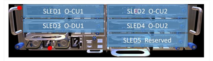
Figure 4. EP100 sled allocation.
